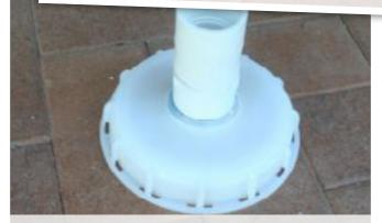
Fittings installed in the lid of the IBC
