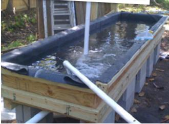
Pumping from the sump tank into the bed with the giant pump
