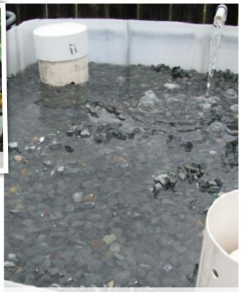
Growbeds fill in around 22 minutes. Worm feeding station at one end and siphon at the other
