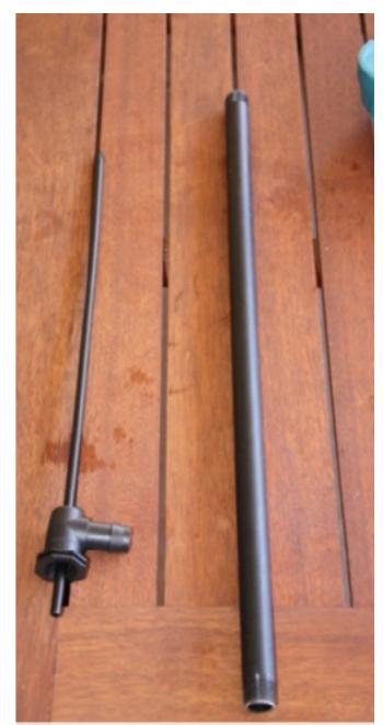
Venturi, all made from reticulation parts
