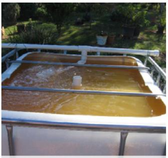
Fish tank showing water return elbowed to create current
