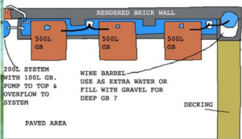
ALWAY! Design showing the IBC growbeds and layout of the custom built fish tank.
