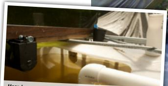
Here is a new input pipe from the sump tank to the fish tank as we felt having just the 90 at the end didn't stir things up enough
