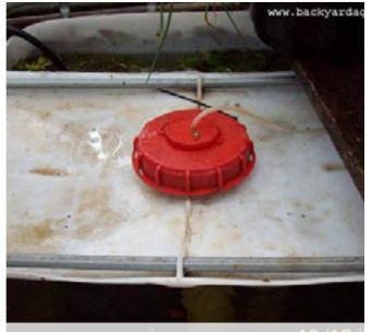
Buried sump tank with air hose dropping down through the lid
