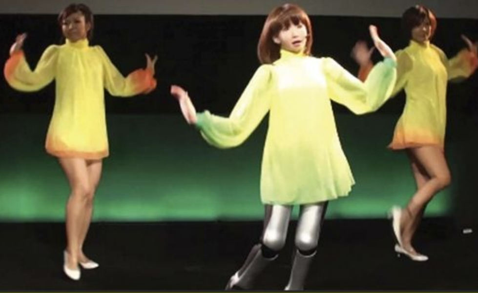
HRP-4C, an android, actually danced and sang on-stage in a chorus line routine with real human dancers as backup. The android is build by Kawada and AIST, of Japan.
