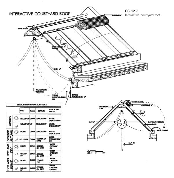
method of evaporative cooling will supplement a conventional evaporative cooler and, in the hot-humid period of July to August, would give considerable cooling when evaporative cooling is no longer effective. The operation of the roof component: chick, water, razai, is to be adjusted from winter to summer and for day and night. The roof provides for:
