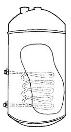
**9.4.** Heat exchange coil in the bottom of a hot water cylinder.
