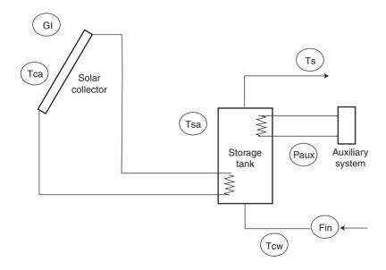
**9.5.** A schematic diagram of the DHW system at the Oxford Ecohouse.
