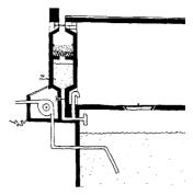
**CS 5.10.** Rainwater harvesting. Section showing in situ sand filter.
