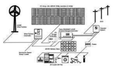
**CS 21.4.** Power supply from the wind turbine and photovoltaic array.
