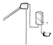
**CS 5.11.** The solar water collector works by thermosiphon.
