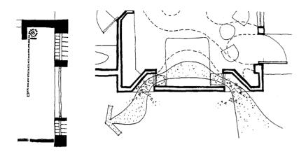
**CS 5.6.** South and west windows, designed to avoid direct solar gain.
