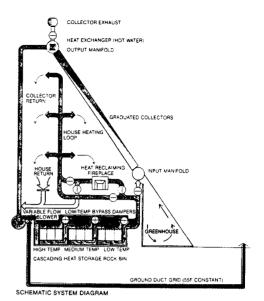
CS 18.7. Schematic system diagram.
