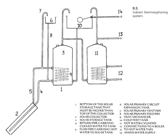
flowing through the collectors from the water flowing to the tap inside the house. It must allow the heat absorbed in the collectors to pass into the water in the storage tank.
