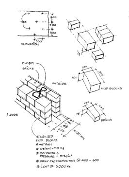
CS 5.4. Wall construction, using stabilized mud blocks (country bricks).
