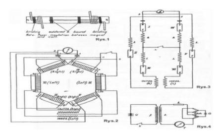
This device consists of six permanent magnets wound in a special way so that the circuit includes the magnet itself as well as the winding. (See Fig. 1).
