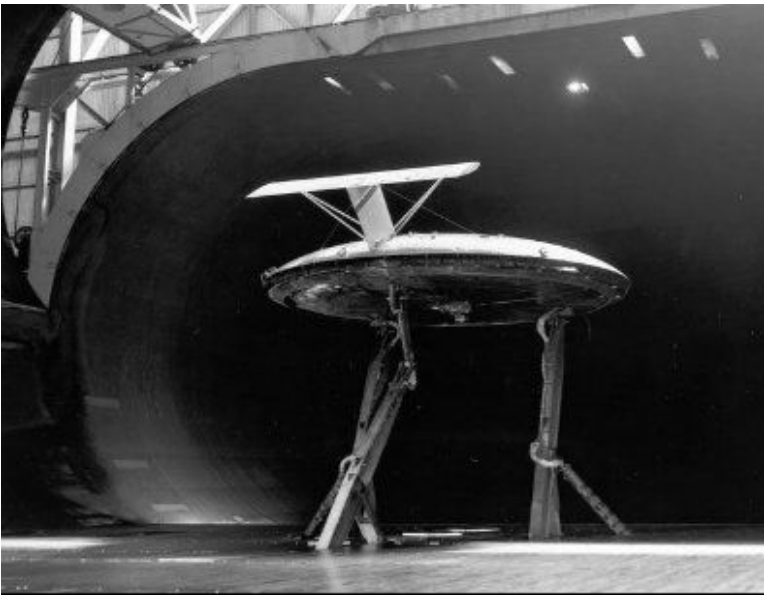
Figure 17: AVROCAR. This Avrocar photo was not taken at Wright Field; it shows the vehicle ready for testing in the 40 x 80 feet Ames Labs (Cleveland, OH) subsonic wind tunnel. According to the rumors and hearsay, the Figure 17 photo supposedly showed, "irrefutable proof that the United States had captured extraterrestrial spaceships and stored them in the mythological Hangar 18."
