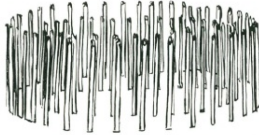
Sticks in double row around the two ovals. This is the appearance of the frame structure for coracle building.
