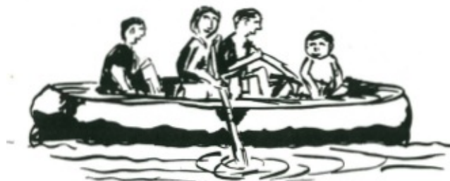
This is a completed coracle launched. A coracle six feet by four wide with fifteen-inch walls will easily support four men.
