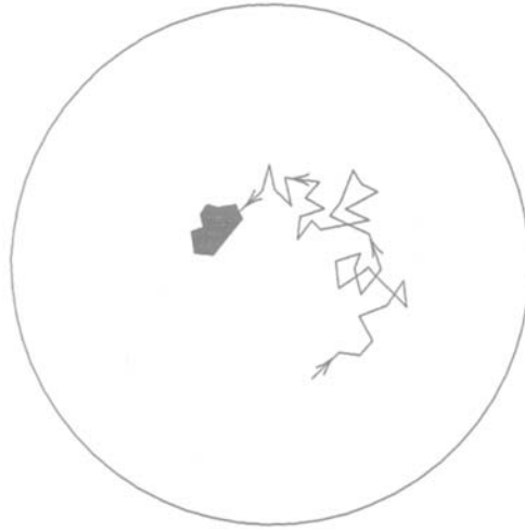
Figure 10.8 Brownian motion: as viewed in a high-power microscope, the particles of smoke suspended in a gas display a ceaseless jittering motion as they are continually battered on all sides by the flying molecules that make up the gas.
