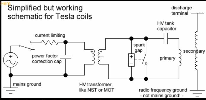
are the bare bones plans for making a Tesla coil. Note that many absolutely essential safety factor parts are not shown, for simplicity of the schematic.
