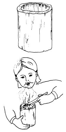
Figure 13-1. Burning out a wooden container.
