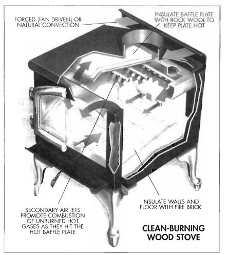
Figure 11-15. Clean-burning wood stove features. Illustration courtesy of Aladdin Hearth Products, manufacturers of Quadra-Fire wood stoves.
