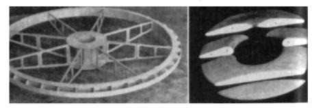
6ft dia. part structure illustrates simple construction of the circular wing.
