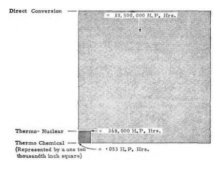
Fig 57. Theoretical energy relationship at the three main levels of exchange, for an expenditure of 1 gram.
