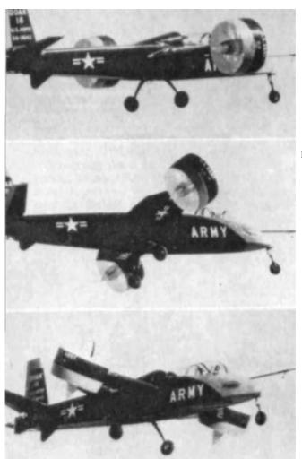
Plate 4. VTOL sequence of the experimental DOAK aircraft with ducted swivel rotors.
