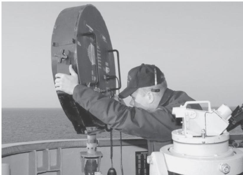
*Long-range acoustical device, developed by the Navy*
