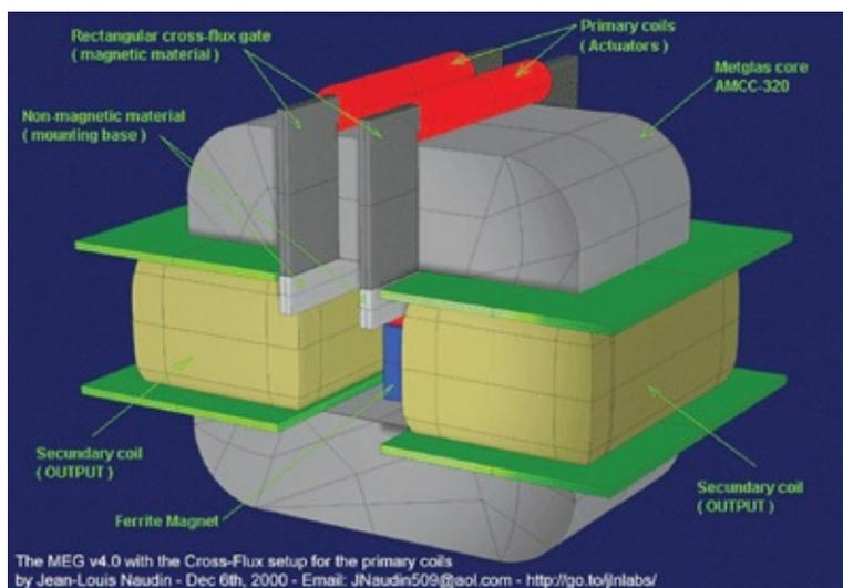
Plate 21. The motionless electromagnetic generator; U.S. patent no. 6,362,718
