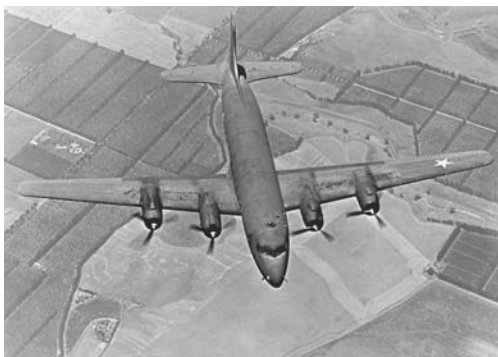
A big C-54. This was the military transport version of the DC-4, the largest airliner of the time. (Author's collection)
