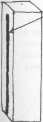
SLOT IS CUT SO THE BLADE WILL FIT EVENLY WITH THE HILT
