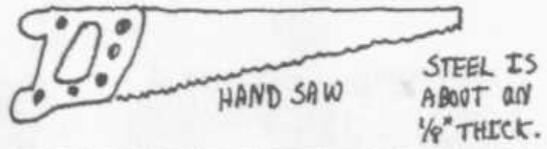
THIS IS A SECTION OF THE CROSS-CUT SAW BLADE. THIS IS WHAT KNIFE BLADE WILL BE MADE OF. THE STEEL WILL BE CUT WITH A COLD CHISEL AND A HAMMER.
