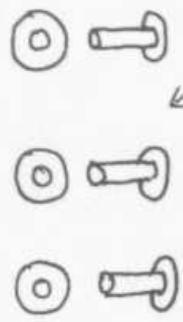
HAMMER THIS SIDE OF THE RIVET. MAKE SURE YOU HAVE A FIRM BACKING. THIS WILL ASSURE A GOOD FIT AND A TIGHT HANDLE
