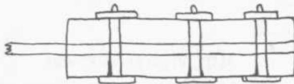
THIS IS WHAT THE RIVETS LOOK LIKE BEFORE THEY ARE HAMMERED INTO THE HANDLE. WHEN THEY ARE HAMMERED IT MAKES THEM SPREAD OUT. THIS CAUSES THE HANDLE TO HOLD FAST TO THE STEEL.
