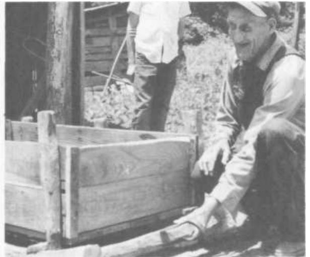
PLATES 193-194 (Variation #4) This sled was made by Harv Reid in Blairsville, Georgia. It has curved sourwood runners and a mortised crosspiece, but the box is nailed to the standards and rests on crosspieces that are nailed to the tops of the runners. In Plate 194, Harv shows where the clevis goes.
