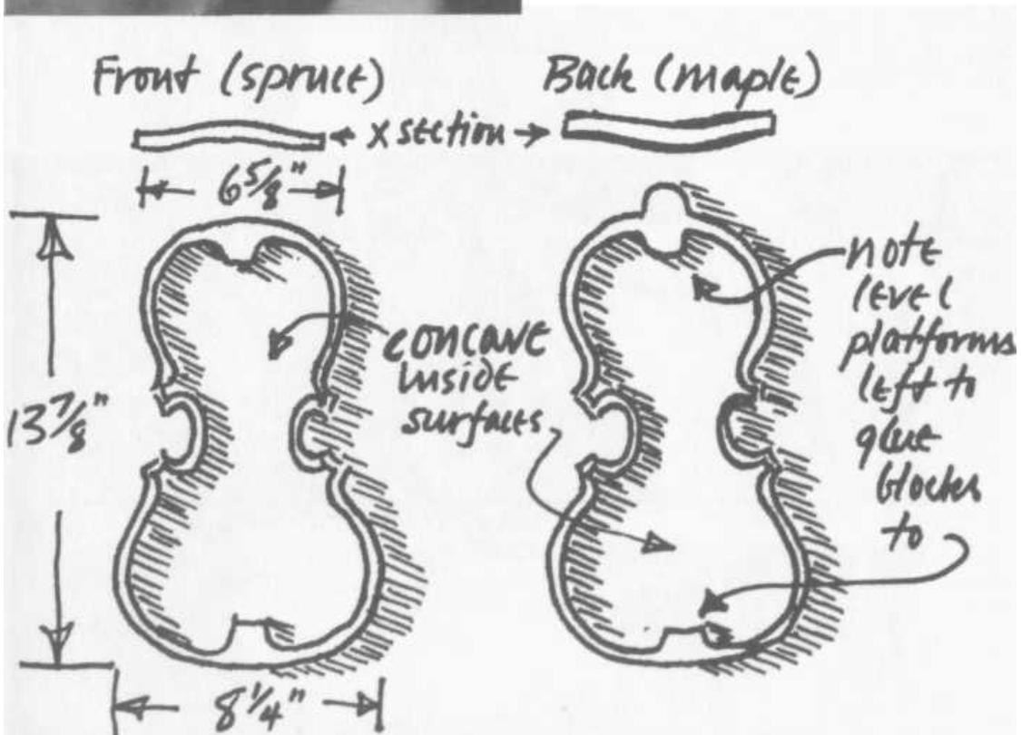
PLATE 112 The patterns used for the fiddle's top and back. These are each made of two pieces of wood  $5/8" \times 15" \times 1/4"$  that are glued side by side lengthwise with Elmer's Glue. (The fiddle is held together only by glue.) The top is made of spruce to produce the be\* sound. All other parts are made of maple (curly maple is best) except the finger board, which is ebony. The diagrams indicate how the top and back should be shaped, and the areas to be "dug out".
