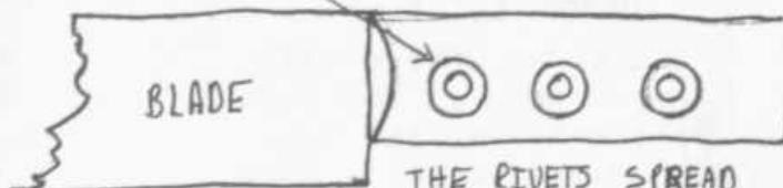
THE RIVETS SPREAD OUT AND HOLD THE HANDLE.
