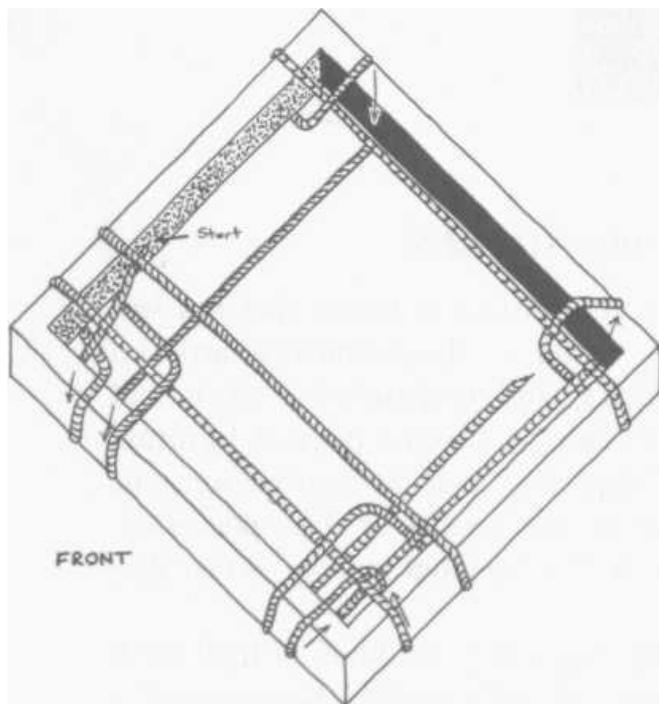
PLATE 413 The pattern for the weave. If the chair you are working on is wider at the front than at the rear (and most will be), measure and build out on the front enough to make the widths equal before starting on the pattern shown.
