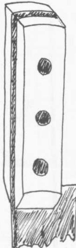
COMPLETED KNIFE AFTER THE RIVETS HAVE BEEN HAMMERED.
