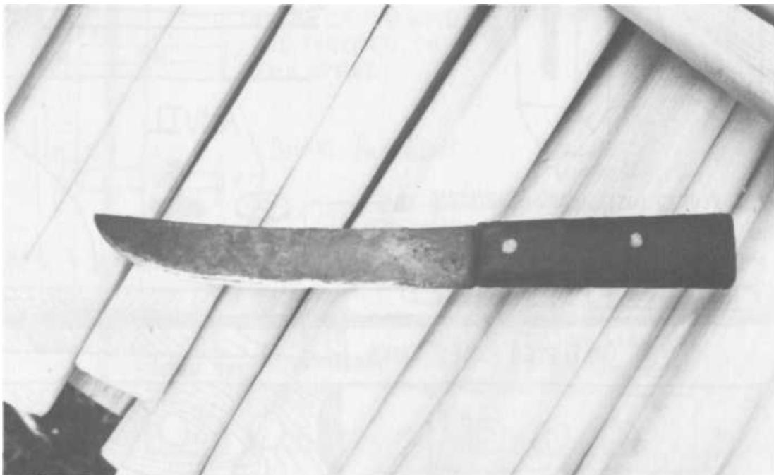
PLATE 39 A butcher knife made by Will Campbell, who died several years ago. He cut the steel using a cold chisel and a hammer. If those tools weren't available, he would warm the steel slightly and scribe a line on it. With the steel hanging over the edge of the anvil, the line on the edge, he would hammer along the line until the excess steel broke off. Like Troy Danner, he usually used old crosscut saw blades for his supply of knife blades.
