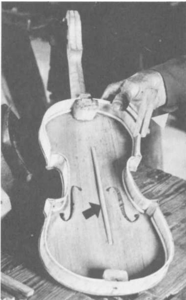
PLATE 120 Overall view of completed top. Note bass bar (dark arrow) which is 7" to 8" long and 1/4" square tapered at the ends. Also note pin holding the lining, as mentioned in Plate 116.
