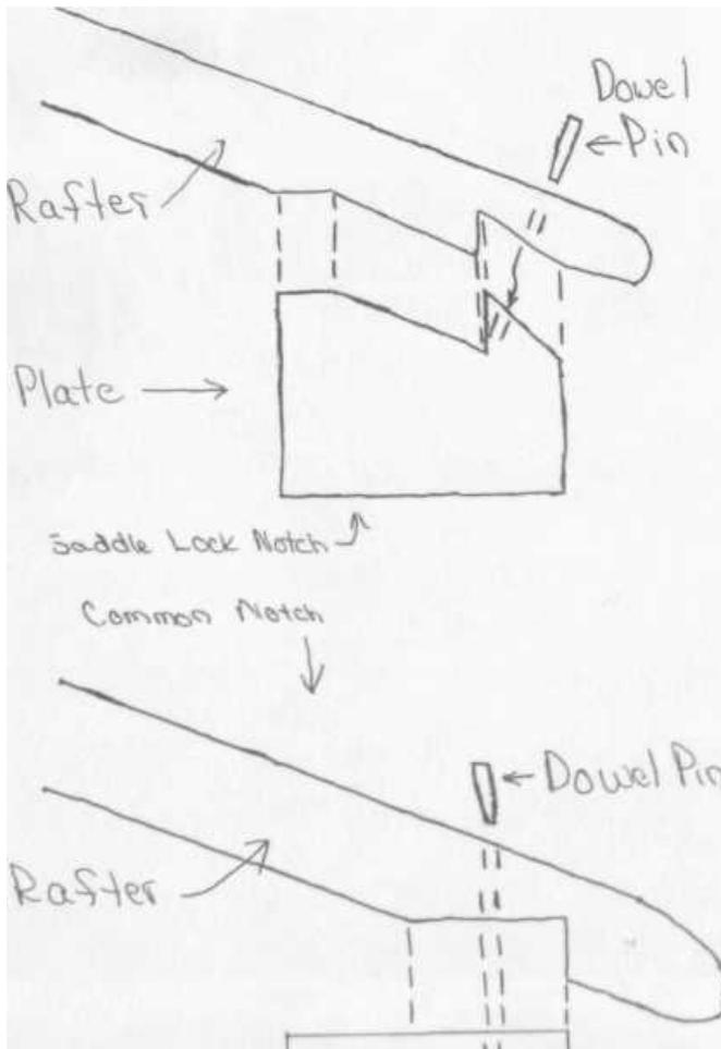
PLATE 411 Two methods of pinning rafters to plates.
