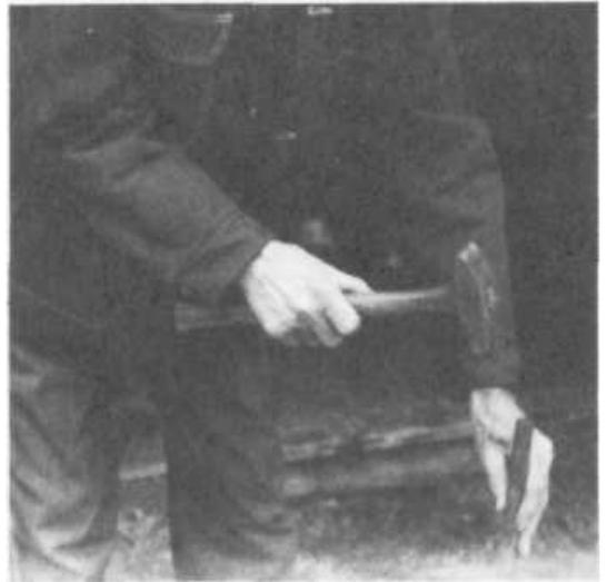
PLATES 33-34 For punching the holes in the blade's base, Troy has fashioned a homemade clamp. The clamp holds the blade tightly while he drives an awl through the blade using the holes in the clamp as a guide. Then he attaches the handle and shapes the blade with a grindstone.
