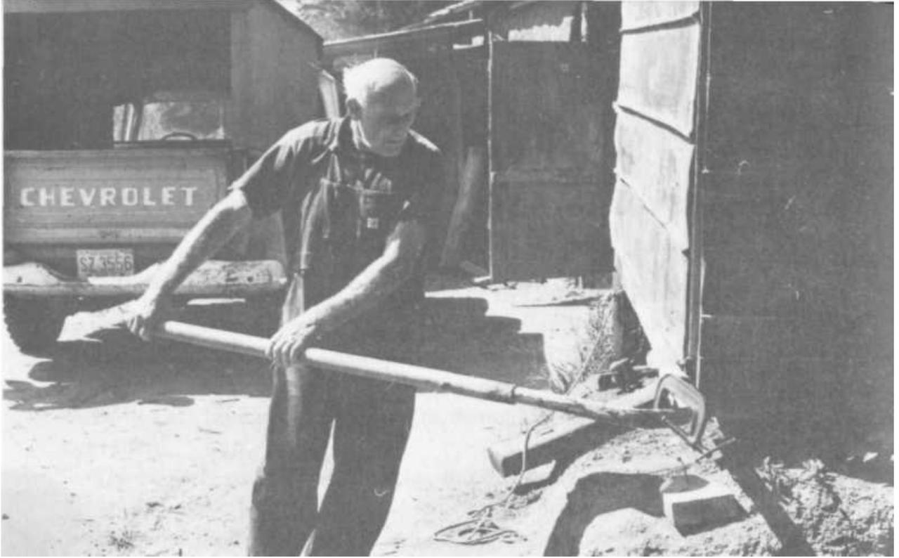
PLATE 443 He then takes the wood to a pipe he has mounted horizontally onto the side of one of his outbuildings. He places one end of the bow into this pipe and the other end into a second pipe which he uses to pull with. As he pulls the section of hickory into an arc, it splits a little as is normal. At the point where it begins to split, he attaches a "C" clamp to help keep it from splitting any fmther.
