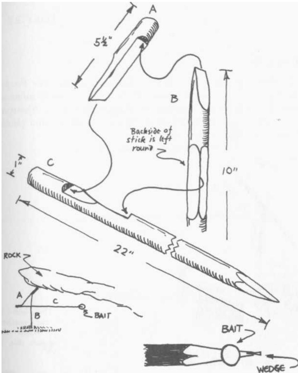
PLATE 229 Dimensions and mechanism of the deadfall.
