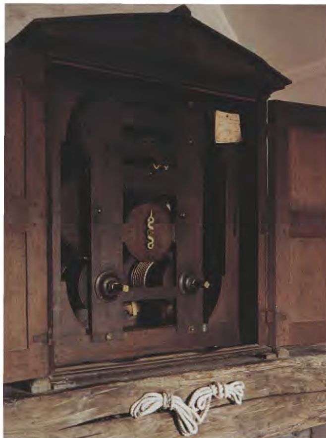
The Brocklesby Park tower clock is housed in a finely made wooden cabinet in the loft above the stables. All the bearings are made of lignum vitae , a naturally oily hardwood that allows the clock to run without any lubricant. The escapement is the first version of Harrison's virtually friction-free escapement, the "grasshopper" escapement, so called because its action resembles the kicking of the hind legs of this insect.
