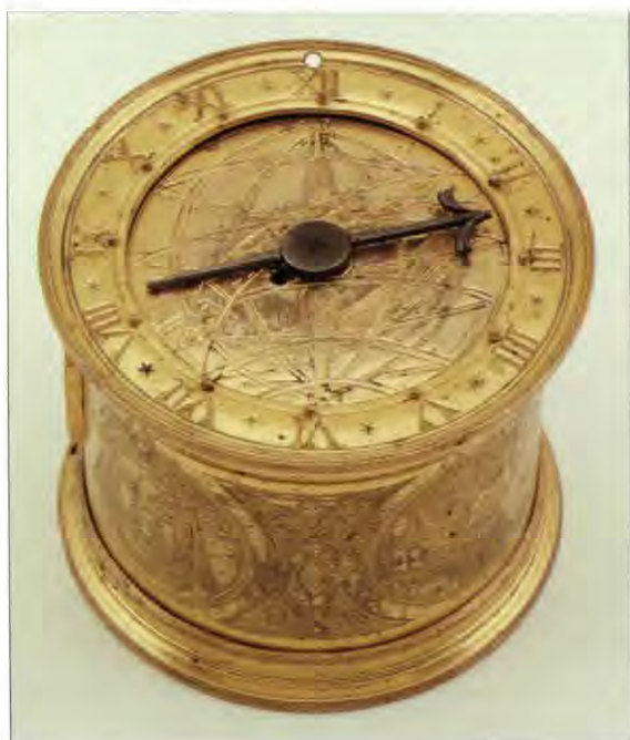
Small, portable, mechanical timekeepers like the one shown here were in use at the time that Gemma Frisius suggested his method of finding longitude. They were usually suspended from a cord attached to a belt or worn around the neck; the drum shape of this example, about two inches in diameter, would have been inconvenient to carry, but in any case these timekeepers were far too unreliable and inaccurate to be of use for navigational purposes.
