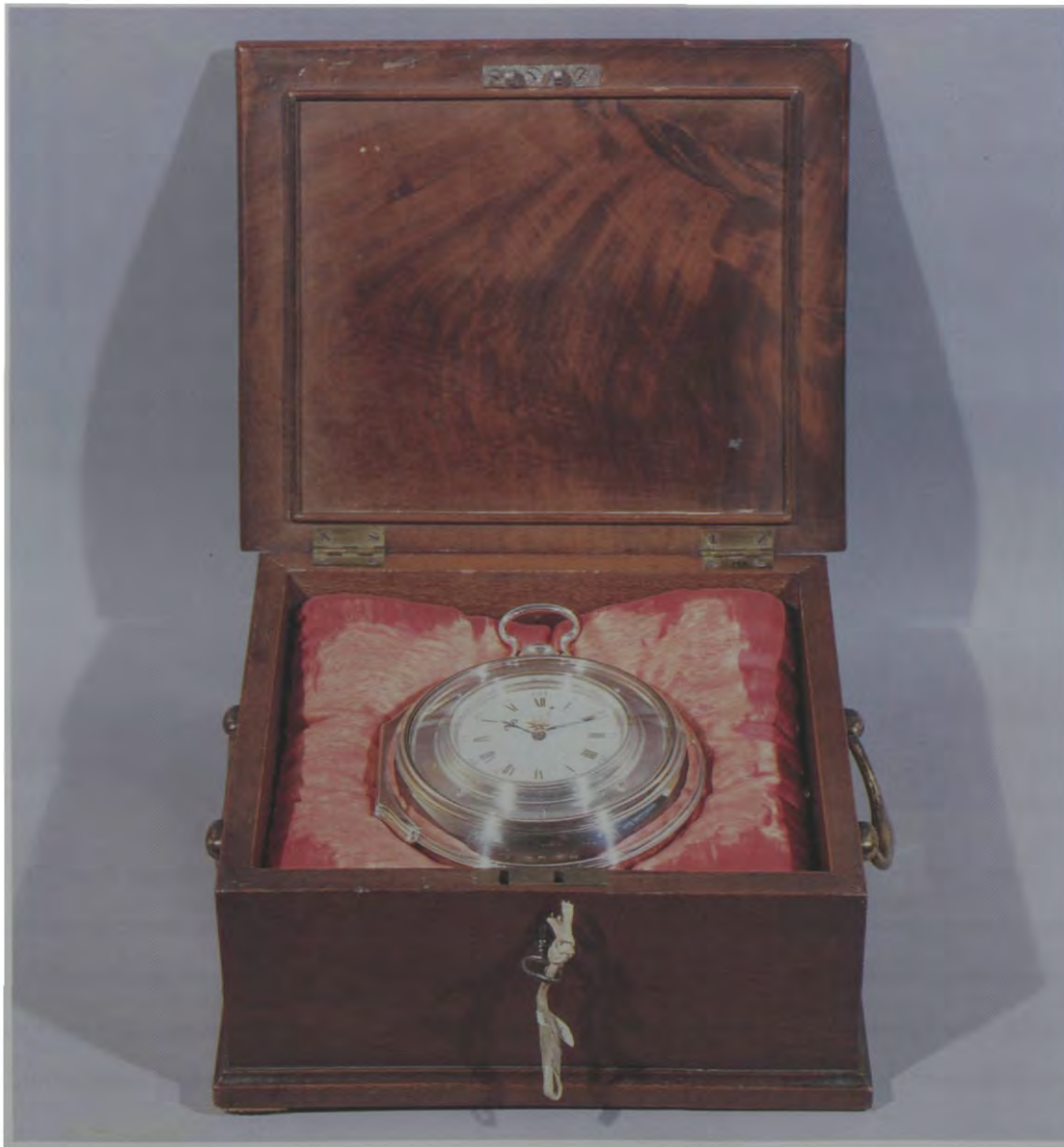
H-5, Harrison's fifth marine timekeeper, shown here in its original box, represents a further development of his work on marine timekeepers rather than being simply a duplication of H-4.
