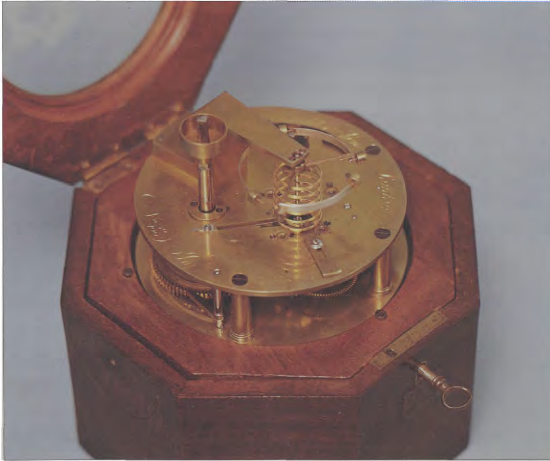
The movement of John Arnold and Son chronometer No. 52/122 is fitted with a gold belical balance spring and Arnold's "YZ" nonferrous bi-metallic balance. Arnold used these materials to overcome the problems of rust and magnetism.
