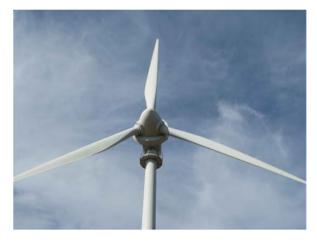
**Fig. 9.5** A gearless horizontal type 500 kW W/T Source: CRES
