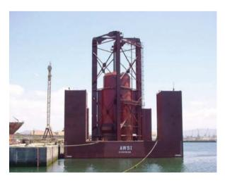
Fig. 9.17 Archimedes wave swing
