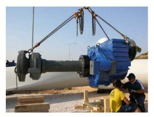
**Fig. 9.4** View of the gear box of a W/T Source: CRES
