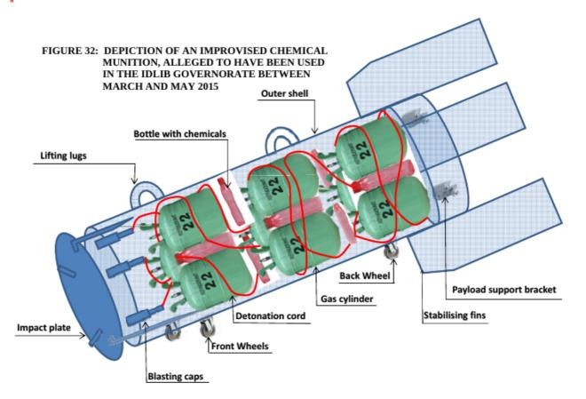
The FFM's reconstruction of the alleged permanganate barrel bomb: Figure 23, Annex 2 page 83 in the report
