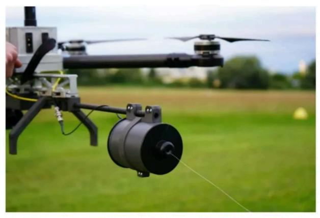
Russia is using drones with the same technology as this German HMX with fiber-optic link rather than ... [+] HIGHCAT
