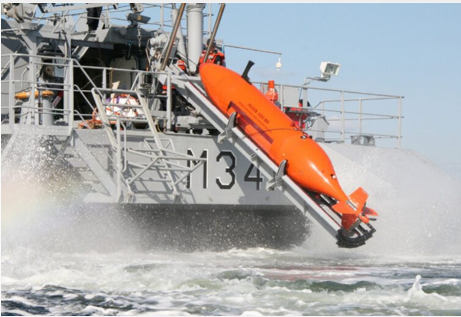
IMAGE: Norwegian Armed Forces testing their new Hugin Autonomous Underwater Vehicle (AUV) from Kongsberg Maritime (source). The Oksøy class M341 Karmøy below was reported to have been scrapped prior to 23 July 2022.
