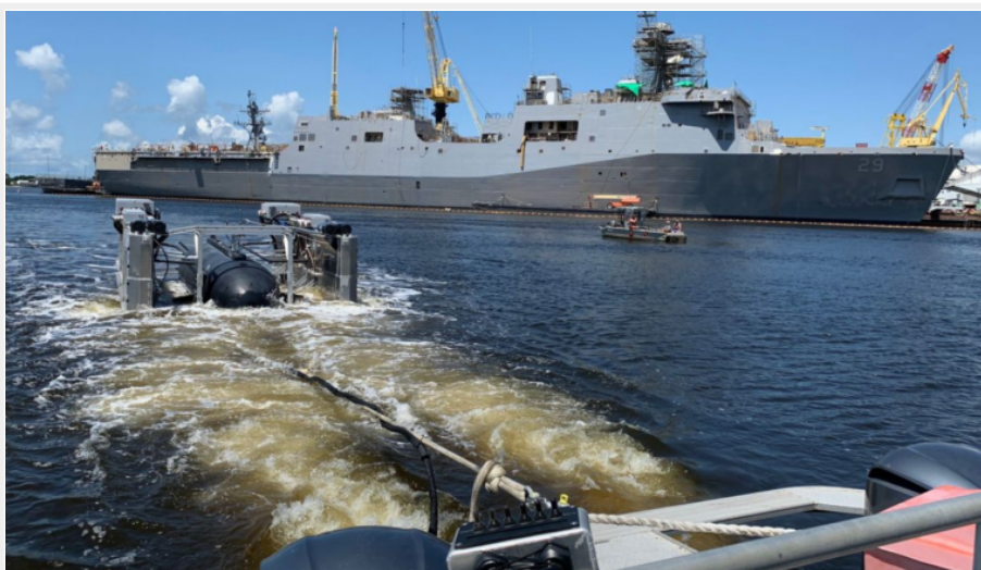
IMAGE: HII's Pharos prototype platform being towed behind a small craft in the Pascagoula River while recovering HII's Proteus LDUUV.
