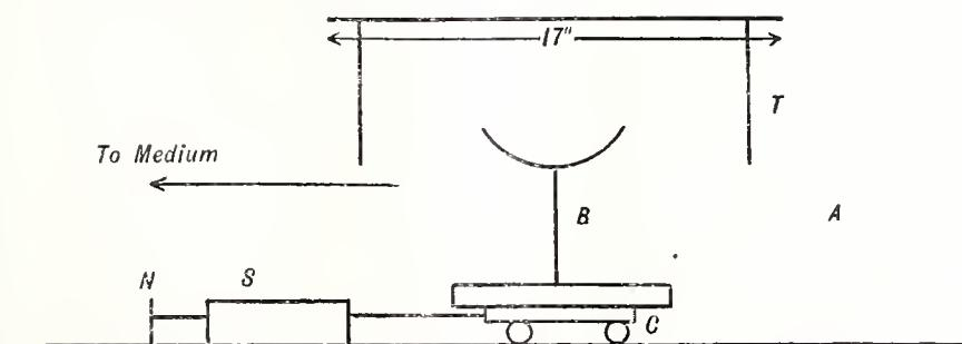
. . . B is the compression balance (reading to 14 lb.) placed on top of an iron carriage C, which runs on ball bearings, and which is so free from friction that a force of  $\frac{1}{10}$  lb. suffices to pull it along the floor. N is a nail driven into the floor. S is an ordinary Salter tension spring balance reading to 20 lb., tied to the nail N and to the carriage C. T is the levitated table. Between A and N is my approximate position of observation.
