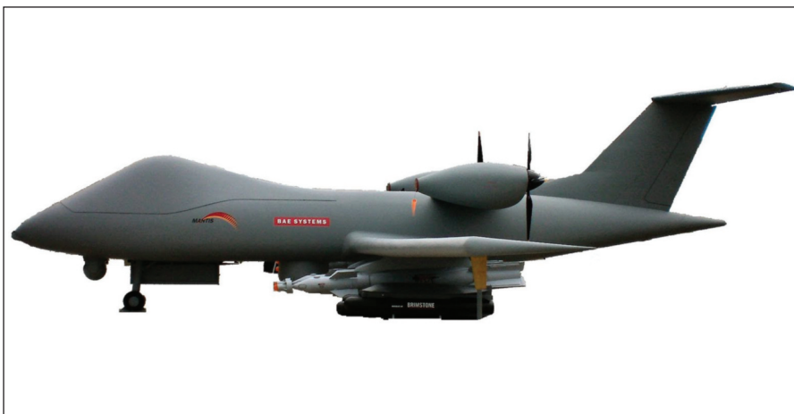
The BAE Systems Mantis, the world's first unmanned autonomous aircraft, i.e., able to pilot itself and to plot its own course. The prototype first flew on 21 October 2009 at Woomera Test Range in South Australia.
