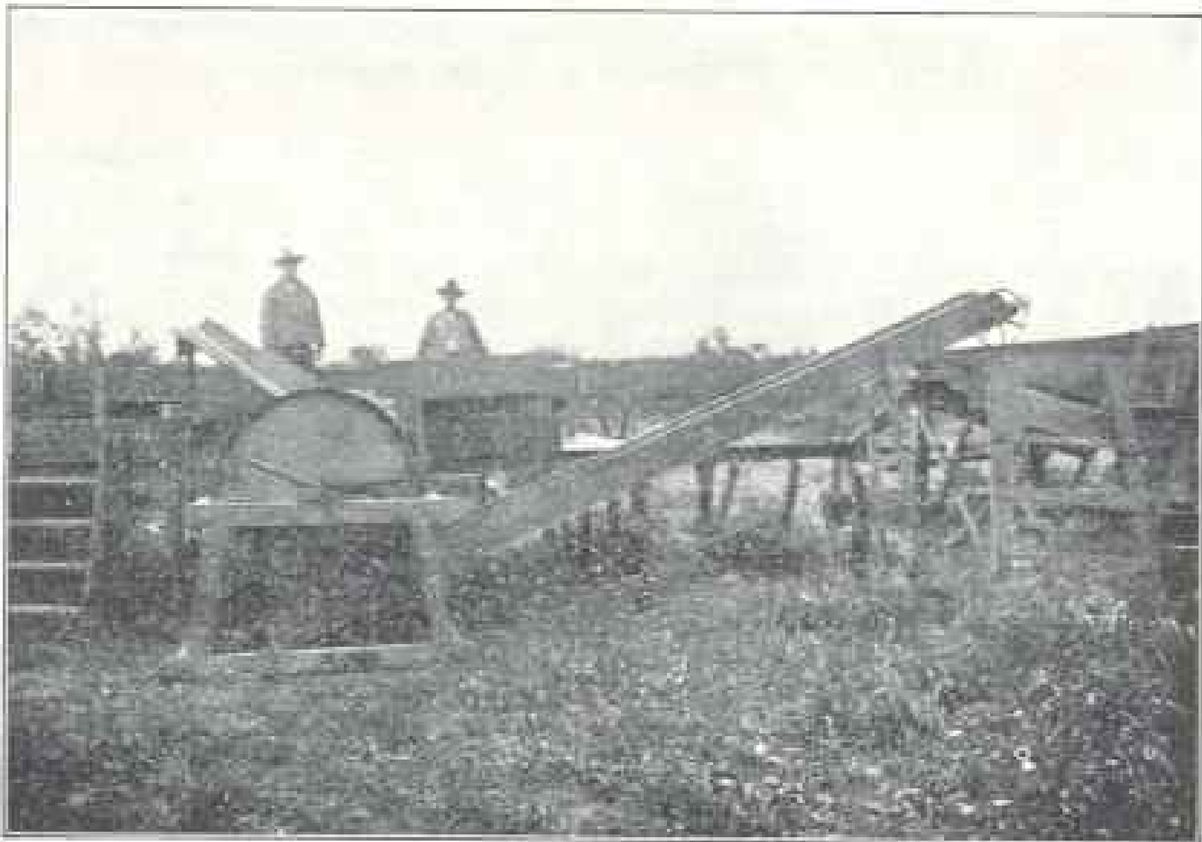
A Type of Pear Cutter, as Set Up and Operated
