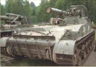
**Self-propelled mortar 2S4 "Tulpan"**
