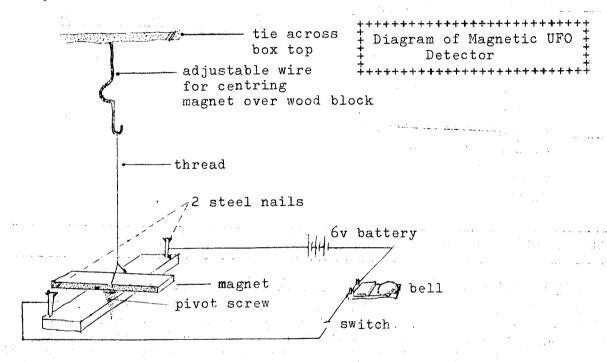
The most suitable magnet to use would be the flat type asillustrated. However, a horseshoe type will be satisfactory if the wooden nail carrier is shortened. Magnets can be obtained from H.W.English, Rayleigh Road, Hutton Brentwood, Essex. The type required should be specified. Short bar magnets can be placed on a meccano strip - after magnetization. Readers who decide to make this detector could look out for magnetic effects during thunderstorms - as these might cause false alarms.
