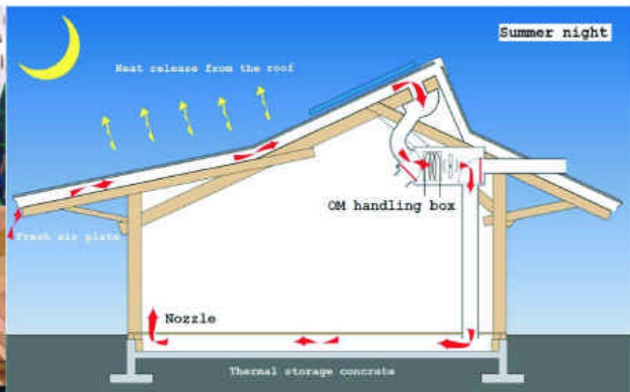
After sunset, the roof releases the inner heat and draws in dry air from outside in to the house. The sensing system senses the room air temperature and the outdoor temperature, and automatically takes in only the cold air under the floor. Here the concrete functions as a cool storage.
