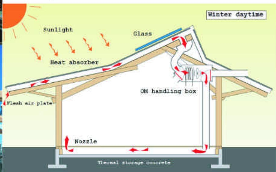
During the winter daytime, the OM Solar system brings down the warm air heated by the roof under the floor, and the concrete absorbs the heat from the air and functions as a floor heater. As the fresh air is always pumped in the room, the room environment will be kept in a good condition. Also in summer, the heat will be ventilated outdoor immediately.
