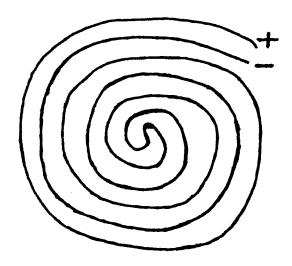
AFTER THE (SENSOR COILS) HAVE BEEN WOUND USING 20 GAGE SPE-AKER WIRE, THIS (BI-FILLER) WINDING SHOULD BE GLUED TO ONE OF THE COPPER TRIANGULAR PLATES ON THE EAST OR WEST WALL OF THE (INNER CHAMBER). WHEN DOING THIS THE (SENSOR COILS) SHOULD BE PLACED BELOW THE (6) POTENTIAMETERS WHICH CONNECT TO THE CIRCUIT. SEE PAGE (17).
