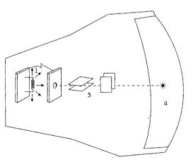
In your TV, the particle source is called a cathode, It's similar to the filament in a light bulb; a little wire you heat up by passing electric current through it, which spews electrons in all directions
