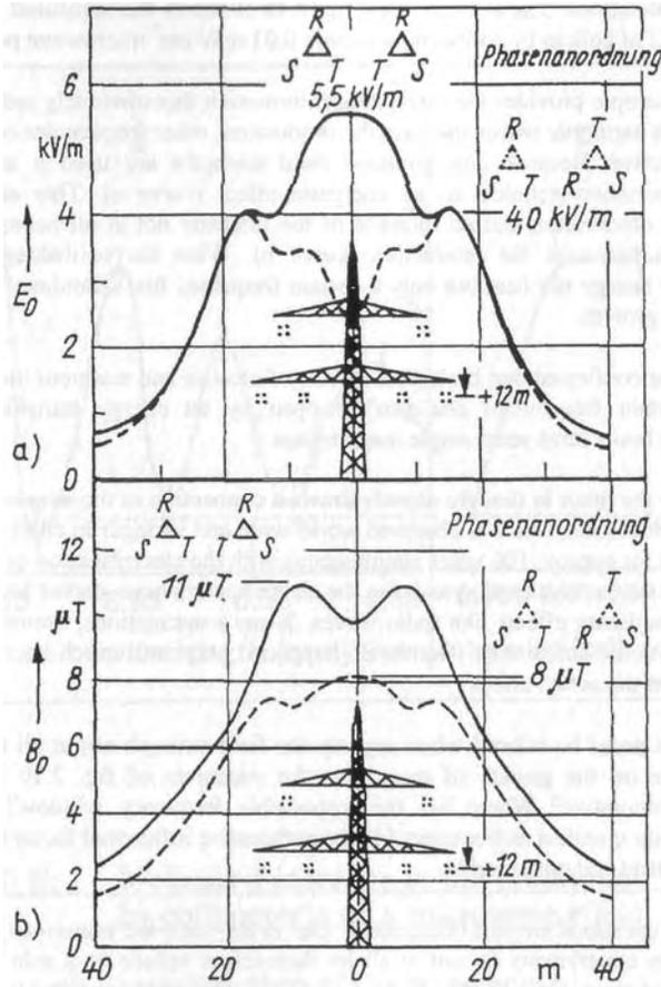
Fig. 2. 11: \_\_\_\_\_ profile of the 50-Hz-field on the ground at 380kV/1kA in each circuit. <i></i>
