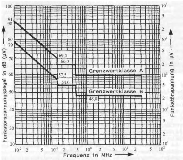
Fig. 2.2: Classes of limits according to VDE 0871
