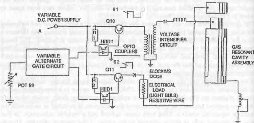
Fig. 17.8: High-tension transformer and driving of the cylindrical water-cell
