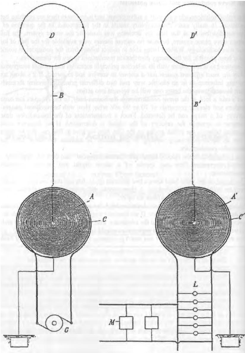
Fig. 9.7: Wireless energy transmission,
