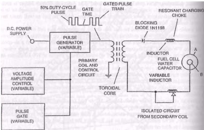
Fig. 17.7: Wiring diagram for the driving of the water-cell<i>
