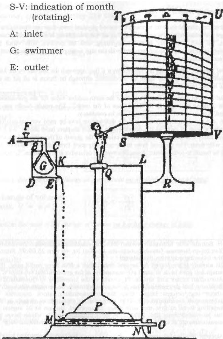
Fig. 13.1: The water meter of the Ktesibios (approx. 250 BC)
