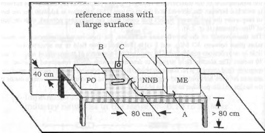
Fig. 2.5: Measurement set up to measure the emission of interferences bound to a conductor.<sup><i></sup>
