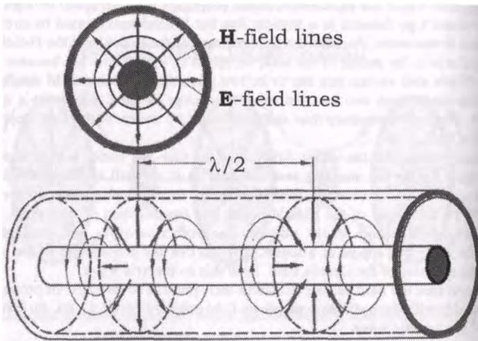
Figure 21.11 B: Wave propagation in a coaxial cable,
