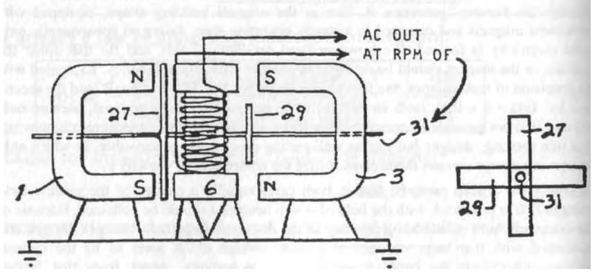
Fig. 16.3: Principle of the Ecklin generator. <i>
