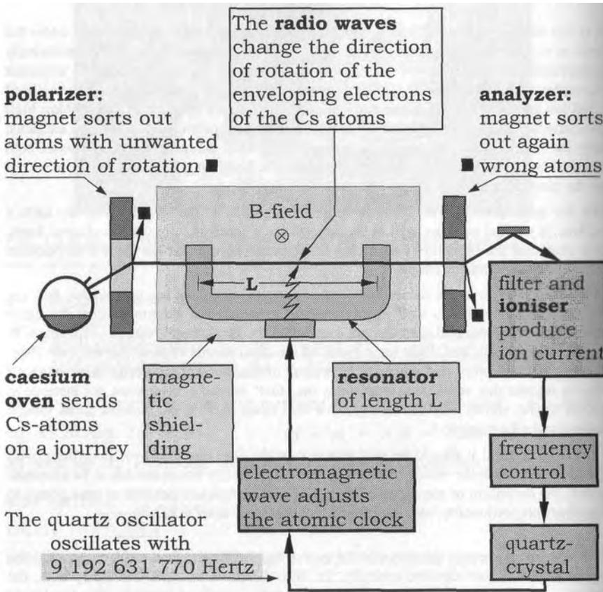
Schematic representation concerning principle of functioning
