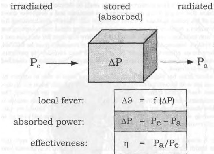
Fig. 1.3: Damping of waves and ability to absorb of a body (our head) if we are making a phone call with a handy.
