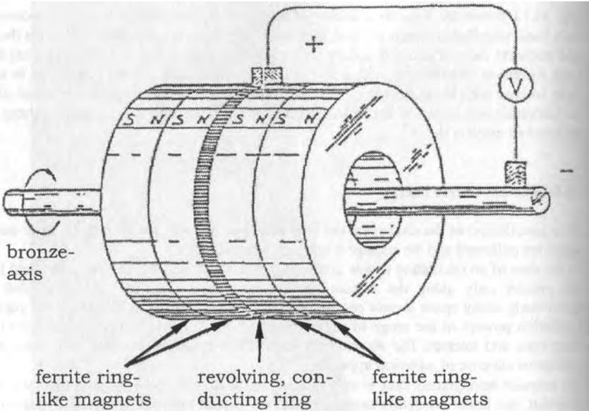
Fig. 16.1: The Faraday generator, which with rotating magnets is called N-machine.<sup><ii></sup>
