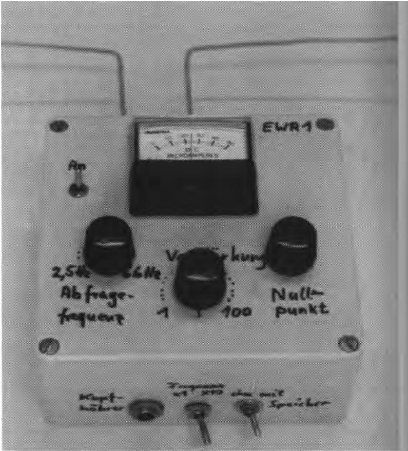
Fig. 19.1: A self-built charge amplifier.
