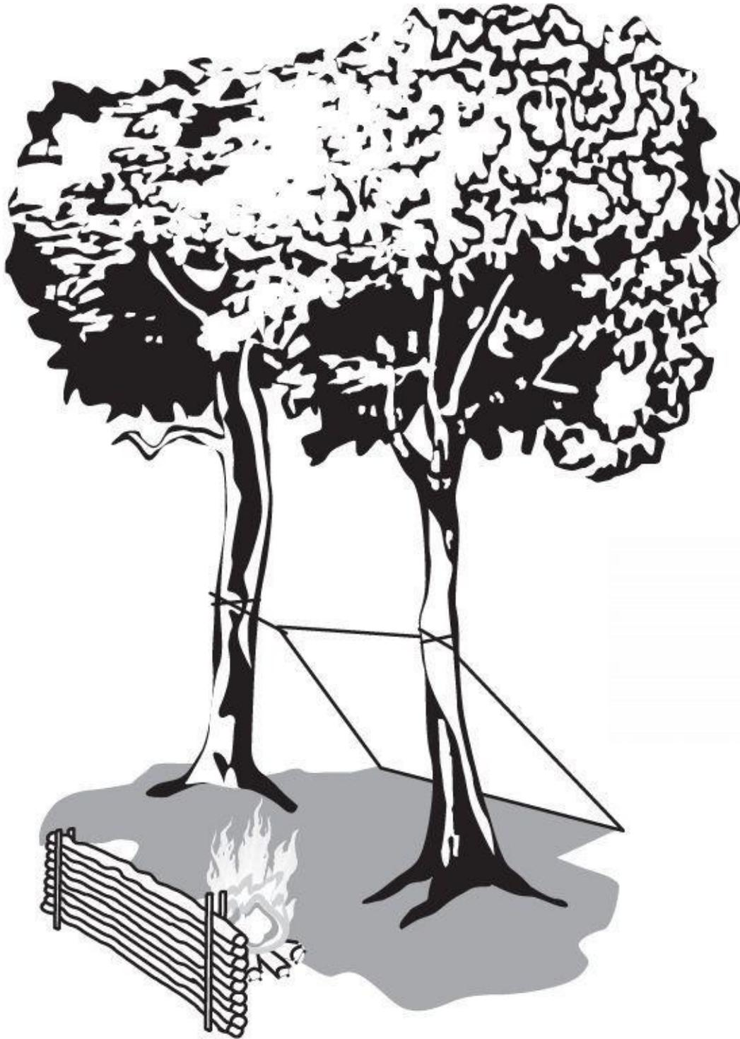
*The reflector fire is one of the best fires for keeping warm in very cold weather.*
