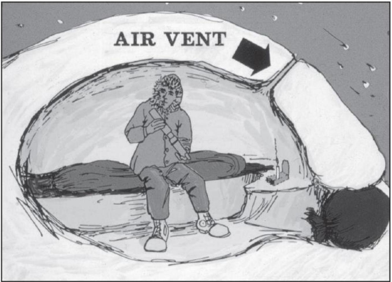
*Constructed in a snowdrift or bank, a snow cave shelter makes effective use of the insulating qualities of snow. The wall should be at least 17 inches thick.*
