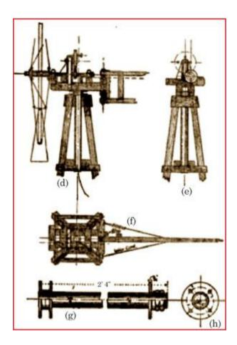
. The windmill turntable (d,e, and f) holds the wheel and tail. The upper flange (detailed drawings g and h) forms a support for the timber framing.
