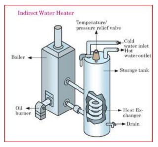
A combination of an indirect water heater and a highly efficient boiler can provide a very inexpensive method of water heating.
