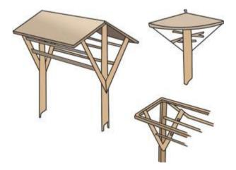
Illustration (a) shows a shelter with a muslin or canvas roof. The inside of the shelter is drawn in illustration (b). Illustration (b) shows a shelter made out of a barrel hoop.
