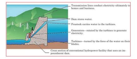
Diagram of a hydropower plant.
