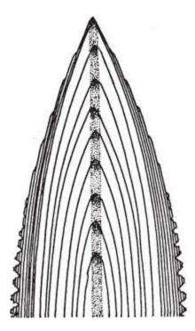
. Fig. 11. Diagram showing the structure of a tree. The dotted part in the center represents the pith. The diagram is of course much wider in proportion to its length than is the trunk of a tree.
