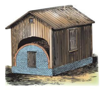
. The drawing shows a common smokehouse that is built on a brick wall and over a brick arch. There are a number of holes left in it for smoke to escape. The ash pit is located beneath the arch, and there is also a door that opens to this pit. To reach the meat room door, use a sturdy ladder.
