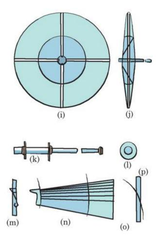
. Details of the wheel shaft frame (i, j); front and side views, (k, l); axle of wheel (m); attachment of inner end of vane to inner ring of frame (n); vane on rings (o); attachment of vane to outer brackets by bracket (p).
