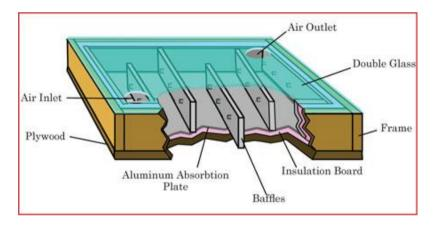
Alternate solar heating panel.
