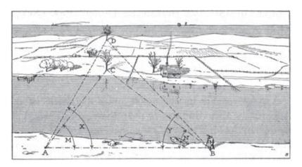
Fig. 110. Determining distances to objects without measuring them.
