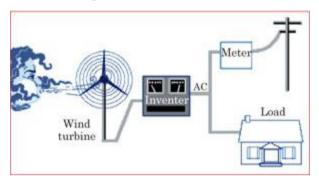
A grid-connected small wind electric system.
