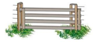
A simple sliding gate can be made for any modern or wire fence.
