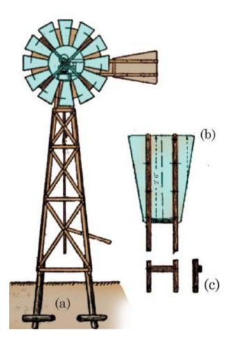
• Details of the windmill. Figure (a) shows a general view with the tail turned to "off" position. Figure (b) shows details of the tail, and (c) shows a cross-piece of the tail.
