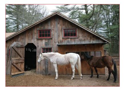
. The Dutch door on this stable can keep animals enclosed while allowing fresh air to circulate.
