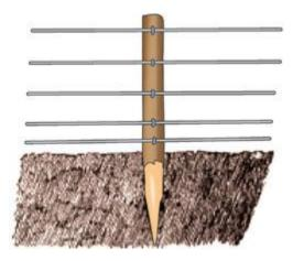
. Drive your fence poles far enough into the ground that they stand firmly upright even when moderate pressure is applied to one side.
