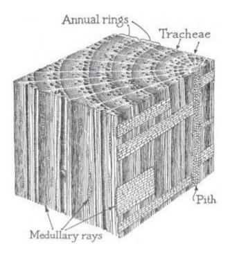
. Fig. 9. The structure of wood (diagrammatic).
