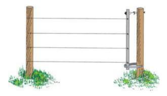
A basic wire gate can be constructed when you need an opening in your fence.
