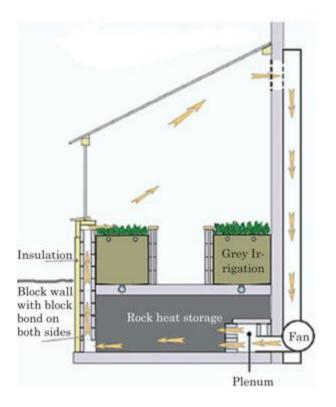
. An active cooling/passive heating greywater irrigated greenhouse.
