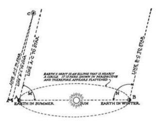
Fig. 112. How the distance to a star is measured.
