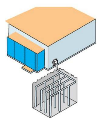
. A vertical closed-loop heat pump system.
