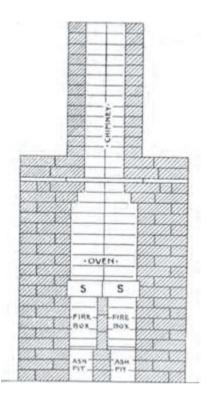
. Cross section of the finished kiln. The space between the walls at the top should not be more than nine inches.
