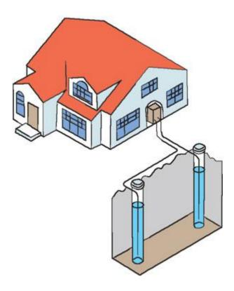
An open-loop heat pump system.
