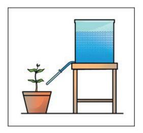
A simple trickle irrigation system.
