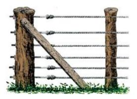
A G-line wire fence consists of three-ply strands of wire.
