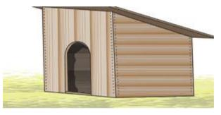
This kennel has a floor that is 2 feet square, is 3 feet 4 inches high in front, and the roof has an overhang of 8 inches.
