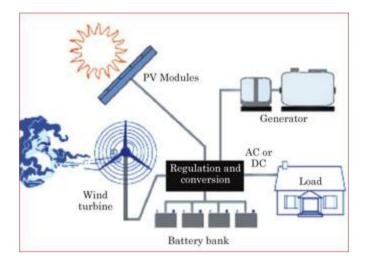
. Hybrid power systems combine multiple sources to deliver non-intermittent electric power.
