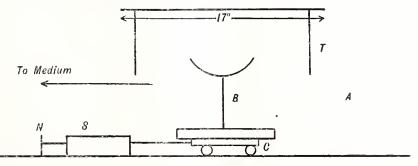
... B is the compression balance (reading to 14 lb.) placed on top of an iron carriage C, which runs on ball bearings, and which is so free from friction that a force of  $\frac{1}{10}$  lb. suffices to pull it along the floor. N is a nail driven into the floor. S is an ordinary Salter tension spring balance reading to 20 lb., tied to the nail N and to the carriage C. T is the levitated table. Between A and N is my approximate position of observation.
