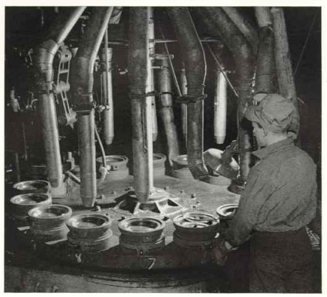
Off a Rotary Press Come Glass Pie Plates Such as Grandmother Never Used An ingenious feeder automatically deposits fiery gobs of molten glass into this turntable press which has 16 molds. Out come Pyrex pie plates. Tubes over each mold are air lines for cooling the glass.
