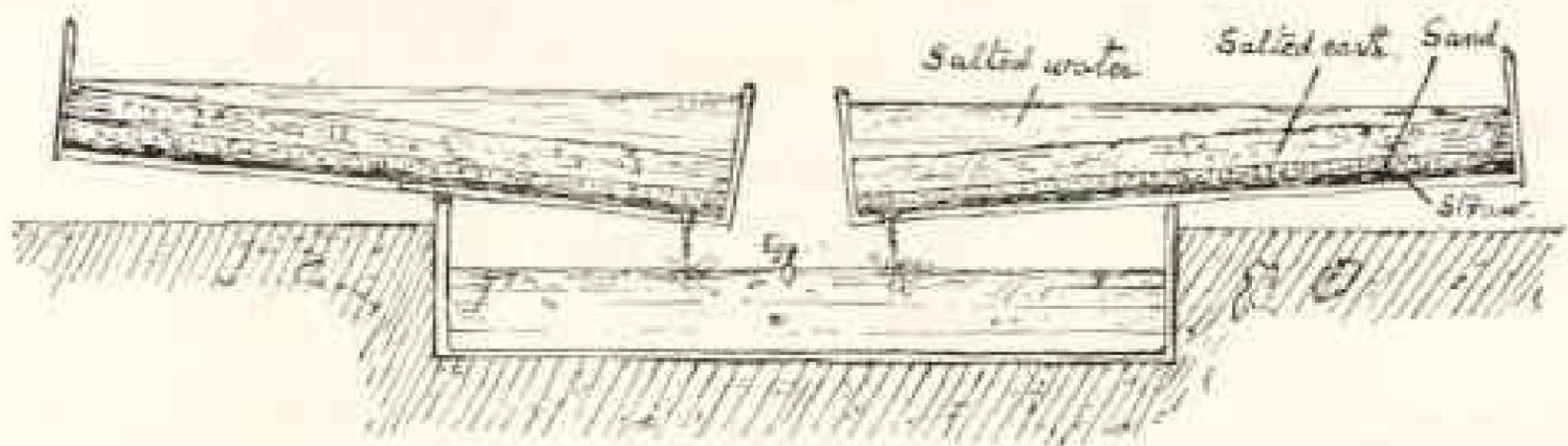
DIAGRAM TO EXPLAIN THE FILTER TANKS
