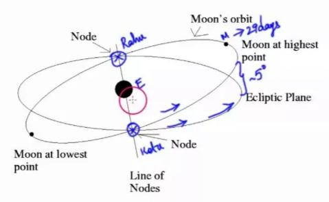
The line of nodes rotates westward 19.4 degrees per year due the gravitational perturbation of the Sun on the Earth-Moon system.
