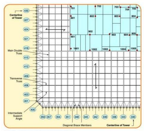
Figure 2-2 Representative structural framing plan, upper floors.
